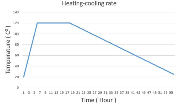
Graph showing the heating and cooling rates applied in the ionic liquid synthesis method.
