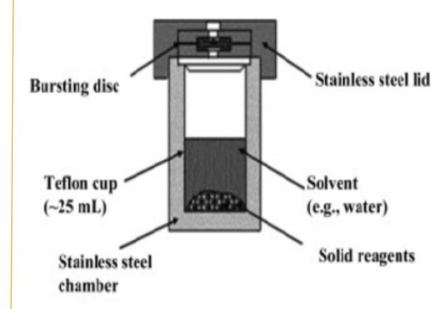
Structure of the autoclave used in the hydrothermal synthesis method.
